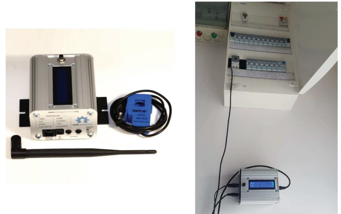
Fig. 1 EmonPi open-source monitoring device with clamp meter and WiFi antenna, and EmonPi installation at household mains supply.
