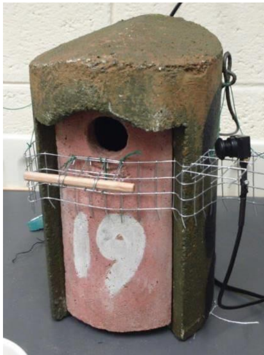
Figure 4.1. The wire perch attached to a nest box with the miniature camera on the left hand side to film the parents coming into the nest box to provisioning their nestlings. The camera was attached to a DVR recorder and a 12v battery. The set-up was placed on the nest box a few days prior to filming to allow birds to habituate. It was placed on day 3 post-hatching in 2017 to record videos at earlier time points (data not used in this study) and on day 15 post-hatching in 2018.
