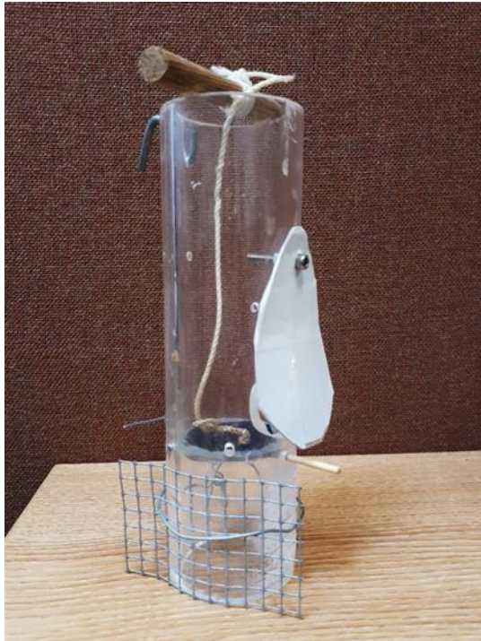
Figure S5.1. Innovative problem-solving device with three solutions. A waxworm is placed on the metal disc in the centre of the tube and a second waxworm is tied to the string that hangs down in the centre of the tube. Birds can either i) push aside the white flap to reach through the hole and take the worm off the metal disc, ii) pull out the cocktail stick lever underneath the flap so the metal disc falls out of the bottom of the tube, bringing the worm with it, or iii) pull up the string from the top of the device to retrieve the worm from the end.
